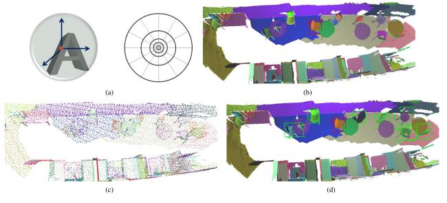
Fig. 5. (a) 3D shape context descriptor. Left: the shape context of a point (in red) can be represented as the spatial distribution in a sphere centered at that point. Right: a 2D view of the sphere. (b) The template (a chair) enclosed by a red box. Each remaining chair consists of multiple regions. (c) The down-sampled point cloud has 20,000 points. (d) Result of the object search: matching objects are found and enclosed by green boxes.
