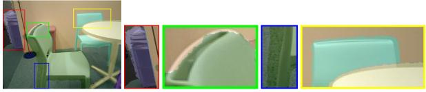
Segmentation by projecting 3D objects into a 2D frame
