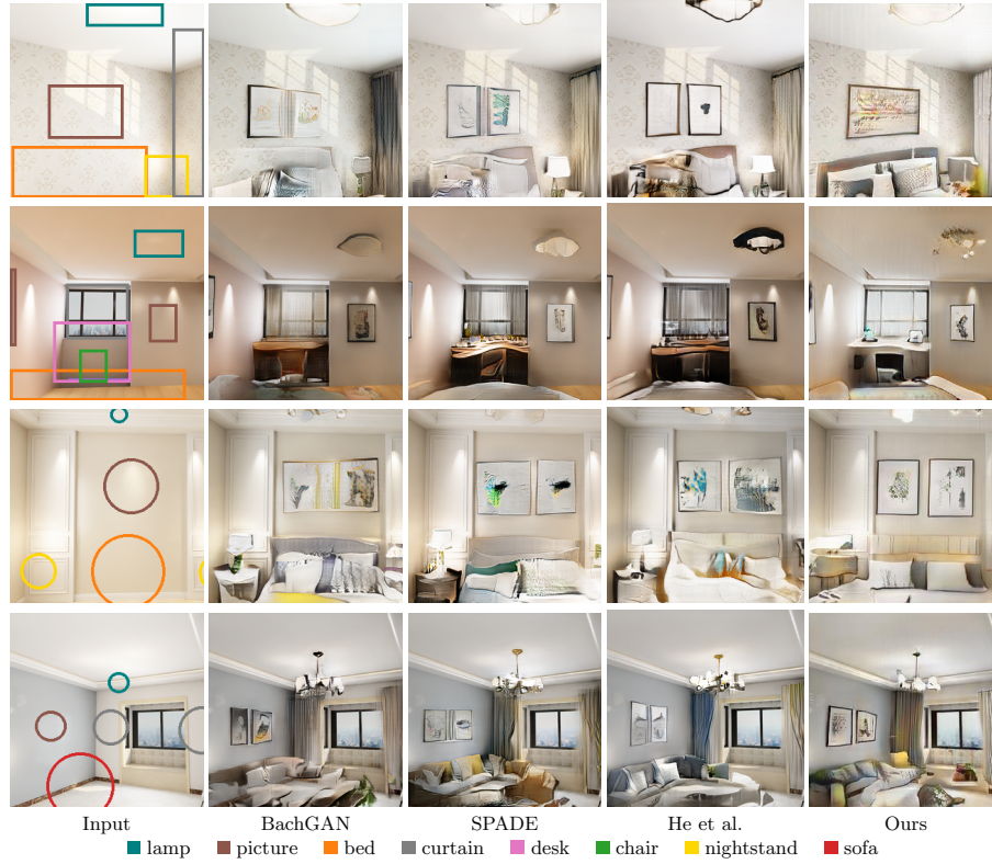
Fig. 2. Generation results of our method and other baselines, using box label format (the first two rows) and point label format (the last two rows). For point label format, the center and radius of each circle represent the location \mathbf{c}_i and size s_i of an object (see Eq. (3)). Best view with zoom.
