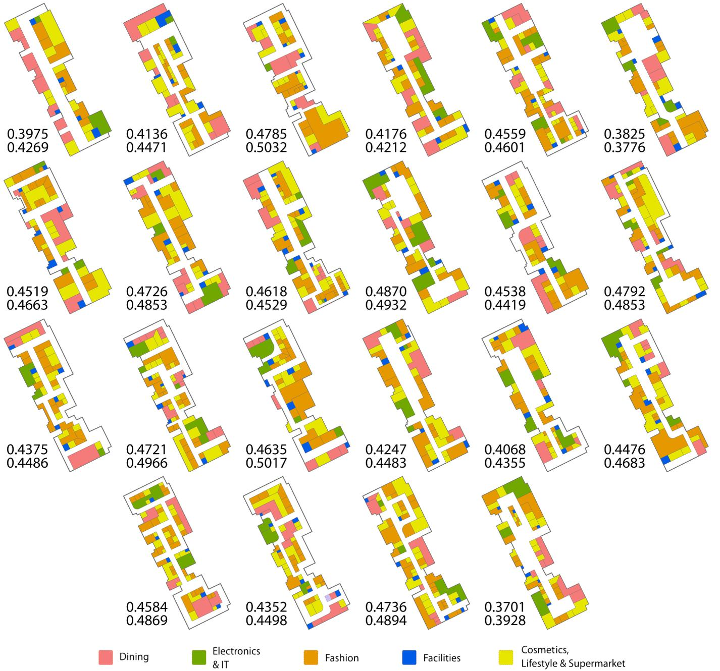
**Figure 5:** User-synthesized layouts of Mall 2. For each synthesis, the numbers at the top and at the bottom are the average crowd densities from AnyLogic and PathFinder respectively. The real world layout of Mall 2 has average crowd densities of 0.8391 and 0.9130 from AnyLogic and PathFinder respectively.
