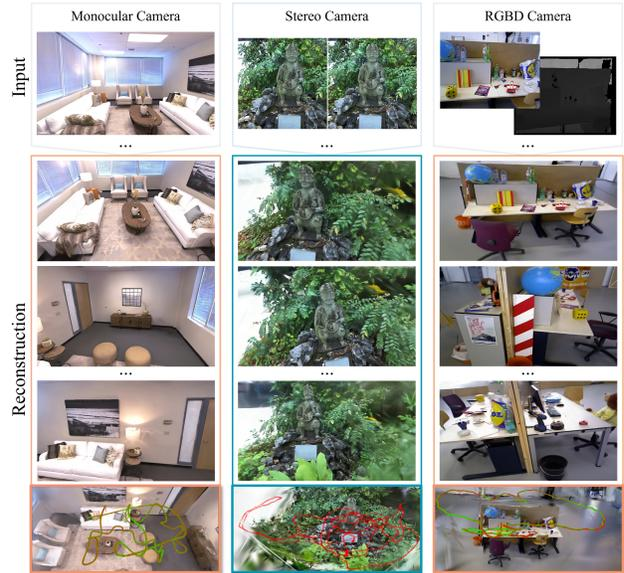
Figure 1. Rendering and trajectory results. Photo-SLAM can reconstruct high-fidelity views of scenes using monocular, stereo, and RGB-D cameras while render speed is up to 1000 FPS.
