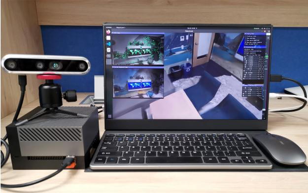
Figure 11. The proposed system has real-time performance on embedded platforms, such as Jetson AGX Orin Developer Kit.
